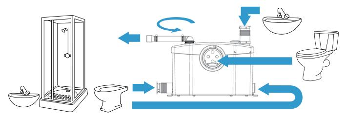
The macerating system of this unit is installed in a case, specifically designed for horizontal outlet spigots. This macerator is manufactured in a factory which is quality certified to ISO 9001(2000) accredited by AFAQ. The correct operation of your unit depends on correct installation and usage.
