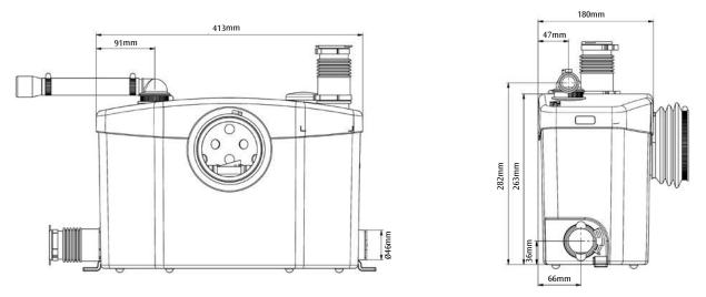
This pump/macerator has been designed to pump away the waste from a WC and the sanitary appliances in step 1.
